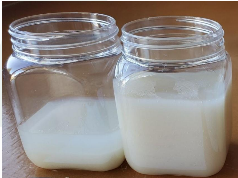
2.5% dispersions magnet stirrer (left) / stick-blender (right).
