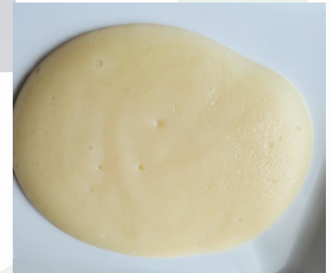
2.5% dispersion, Ultra-Turrax 15,000rpm, 2 min.
