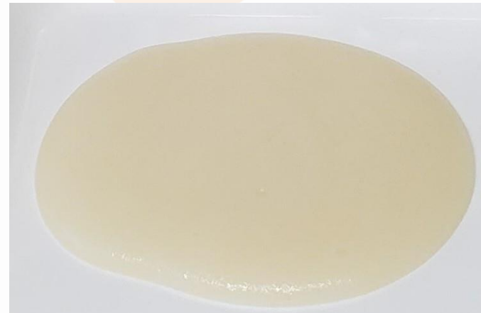
2.5% dispersion, Ultra-Turrax 10,000rpm, 1 min.
